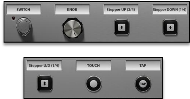
Fig 56 - Smart Controls types: Switch, Knob, Step Up, Down and Up/Down, Touch and Tap
